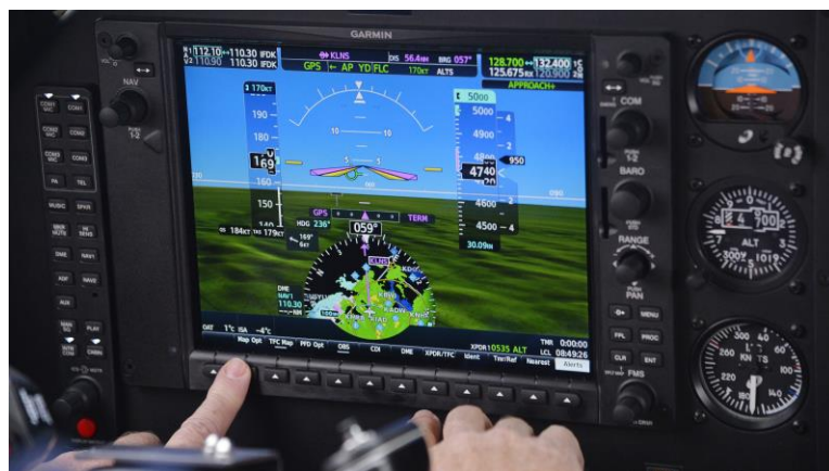
Figure 4 The Garmin 1000 Flight Deck ( https://www.aopa.org/news-and-media/all-news/2017/january/03/garmin-launches-new-generation-of-g1000-cockpit ).
